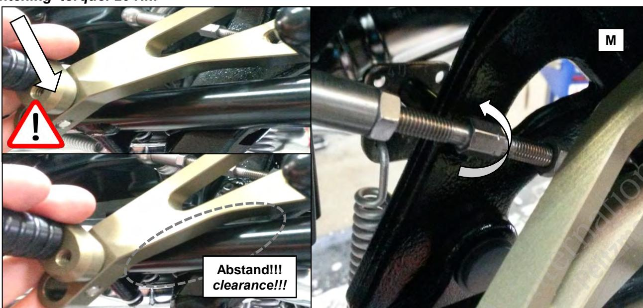
**M:** Pushing the gear lever by hand into lowest position, to check if there's enough clearance to the side stand. **No touching of the lever to the side stand allowed!** Possibly, you need to adjust the lever height by changing the gear shafts setting. Turn it into a higher Position.
