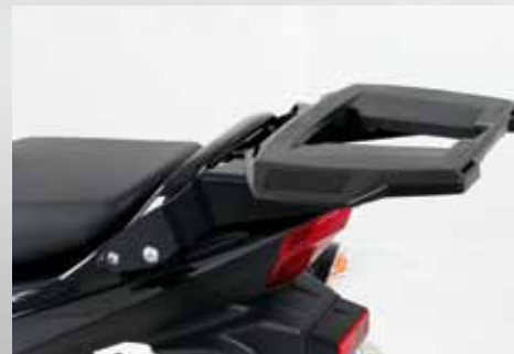
Alurack without bow for carrying luggage
