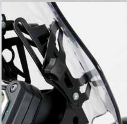
Adjustment for OEM windscreen 420.4531-06
