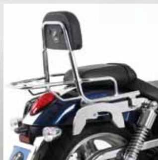
TRIUMPH Thunderbird 1600 Sissybar with Rear rack
