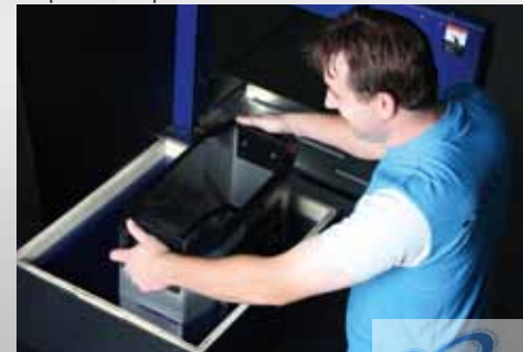
Final leak test
