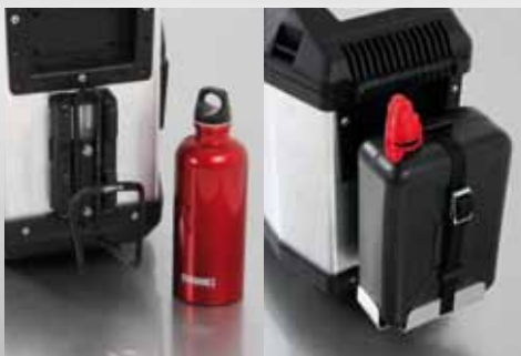
Holder for bottles incl. holder (bottle not included) 2 litre canister with holding plate
